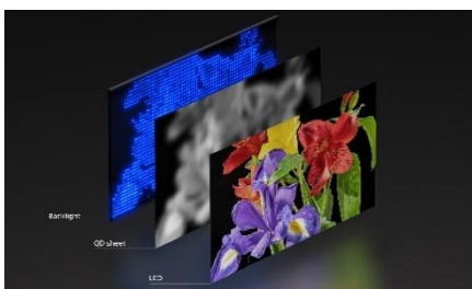
Conventional LED backlight system.
